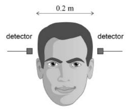
To determine the position where the gamma photons are produced between the detectors, the scanner measures the short interval of time  $\Delta t$  between the triggering of the first detector and the triggering of the second detector.
