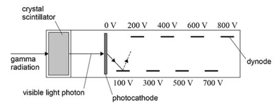
At the crystal scintillator, each photon of gamma radiation leads to the emission of one visible light photon.
